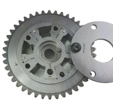
6. Once the internals are accessible, you will see 5 inner vanes that are positioned against the outer portion of the gear. This is where the lockout will be installed.
