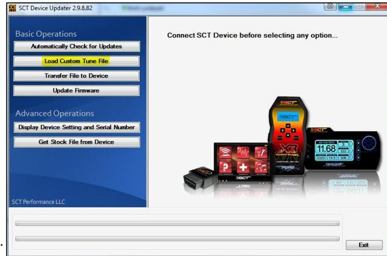
**Step 3:** With your device connected to the PC click “Load Custom Tune File” button in SCT Device Updater to begin.
