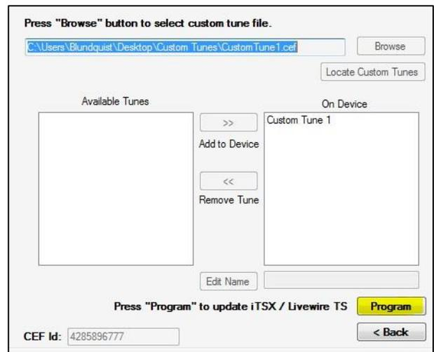
**Step 6.** Now that the tune has been transferred to the X4 (right side), it will appear under “**On Device**”.
